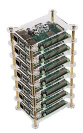
The Maker Case Tower is able to hold up to 7 Raspberry Pis or other expansion boards in the same size. For example, it is suitable to build a server cluster. The acrylic plates and brass spacers are fast and easy to mount.
